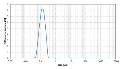
Figure 1: Particle size distribution of CaLoSiL® paste-like
